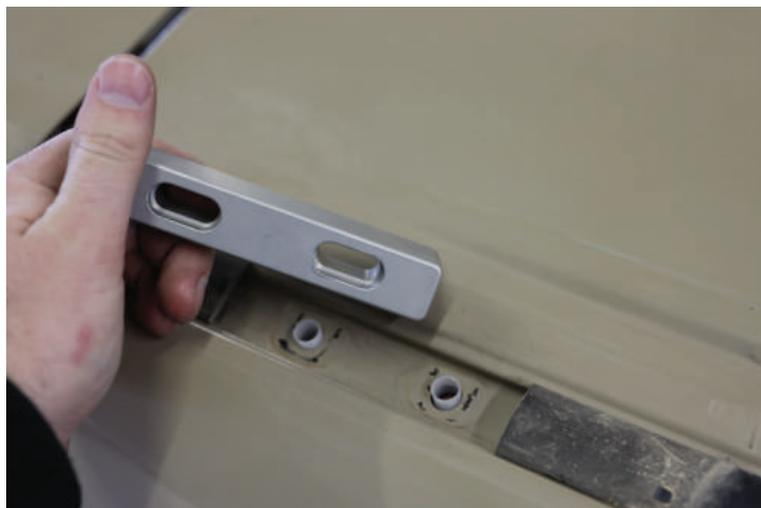
*Attach butyl tape or preferred sealant to interface of the leveling bracket and 4Runner roof track sheet metal.*
